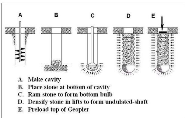
Figure 2 Geopier *Rammed Aggregate Pier*<sup>TM</sup> Construction
