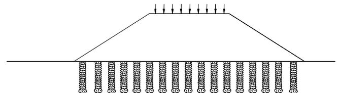
Figure 1 Geopier-reinforced soils beneath embankment
